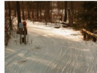
Provide adequate visual cues of an approaching right curve to enhance trail safety. From this direction, the gate and other signs at the trailhead alert the rider of the approaching curve. From the other direction, a warning sign is provided about 100 feet prior to the curve to alert riders to slow down and approach with caution.
