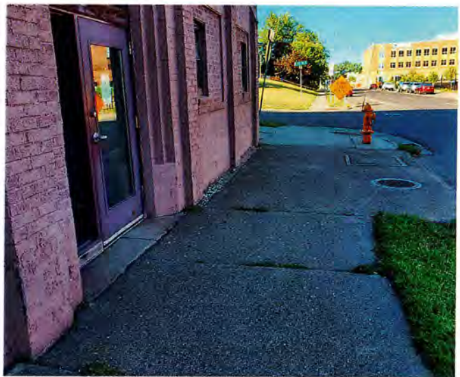
Building entrances require elevation matching – "outside-in" design.
