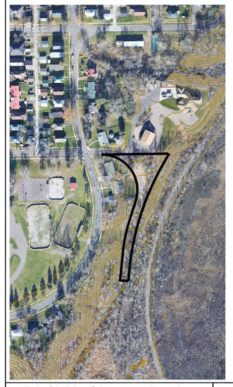
AREA= 0.744 ACRES NOTE: CONTOURS SHOWN ARE BASED ON LIDAR FLIGHT.
