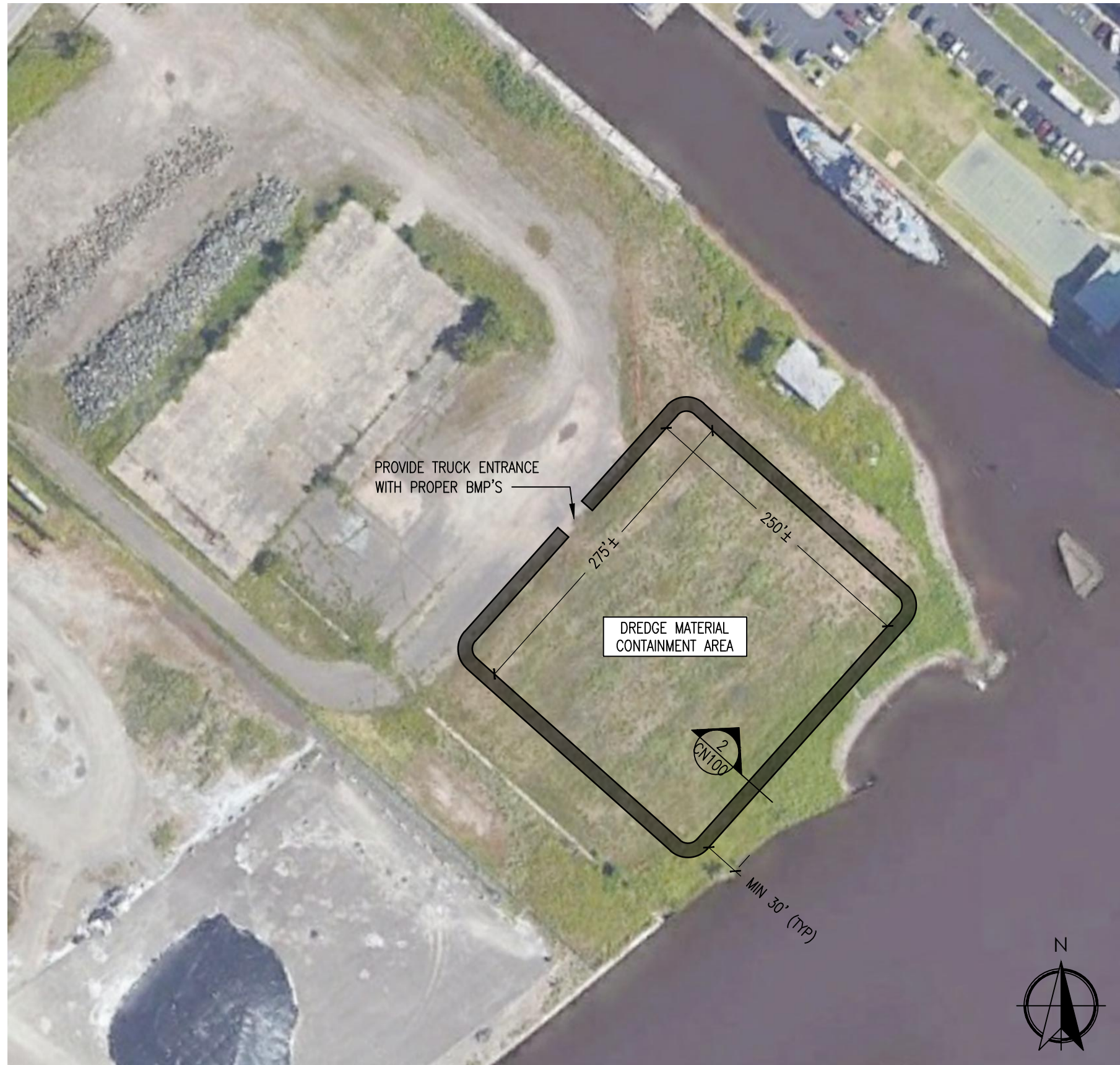
1 DREDGE MATERIAL CONTAINMENT AREA CN101 1" = 100'-0"
