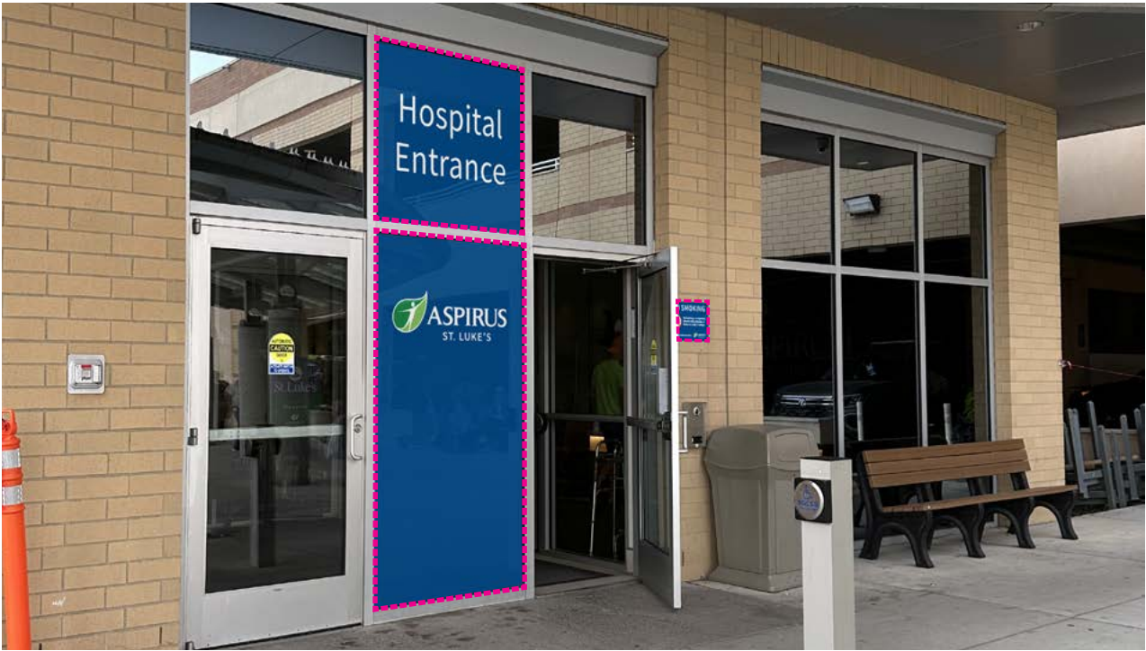
Hospital Entrance Dashed outlined areas above to recieve new printed and cut vinyl graphics. Translucent blue vinyl applied to exterior of glass - VT2 . Cut matte white opaque vinyl applied over translucent blue - V2 . Printed Asprios leaf logo on opaque vinyl also applied over translucent blue vinyl. Replace 'No Smoking' sign with new.
