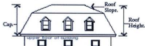
Pitched Roof cap type - Mansard
