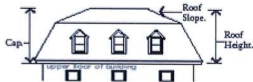
Pitched Roof cap type - Mansard
