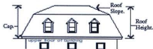
Pitched Roof cap type - Mansard
