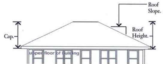
Pitched Roof cap type - Hipped
