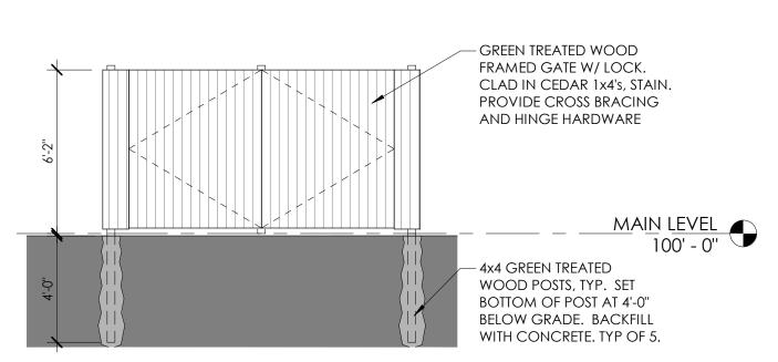
$3 \frac{\text{TRASH ENCLOSURE ELEVATION}}{1/4" = 1'-0"}$
