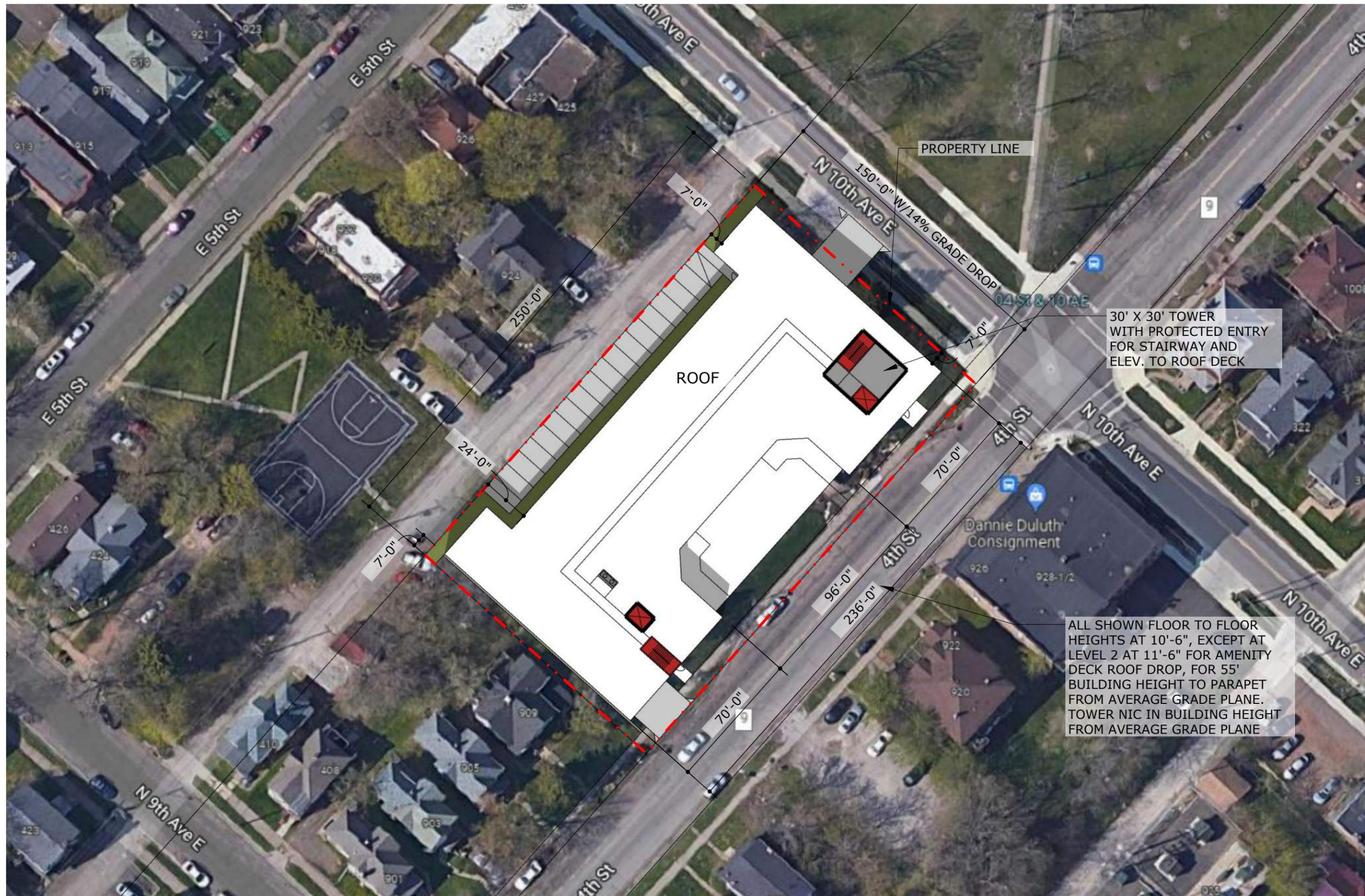
ALL SHOWN FLOOR TO FLOOR HEIGHTS AT 10'-6", EXCEPT AT LEVEL 2 AT 11'-6" FOR AMENITY DECK ROOF DROP, FOR 55' BUILDING HEIGHT TO PARAPET FROM AVERAGE GRADE PLANE. TOWER NIC IN BUILDING HEIGHT FROM AVERAGE GRADE PLANE
