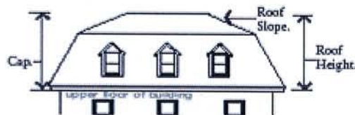
Pitched Roof cap type - Mansard
