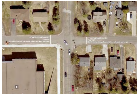
Chambersburg Avenue and Ensign Street. The west side of Ensign is wider than needed.
