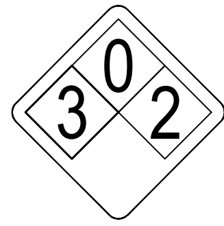
ALERTING SIGN (FOR CELL SITE BATTERIES)
