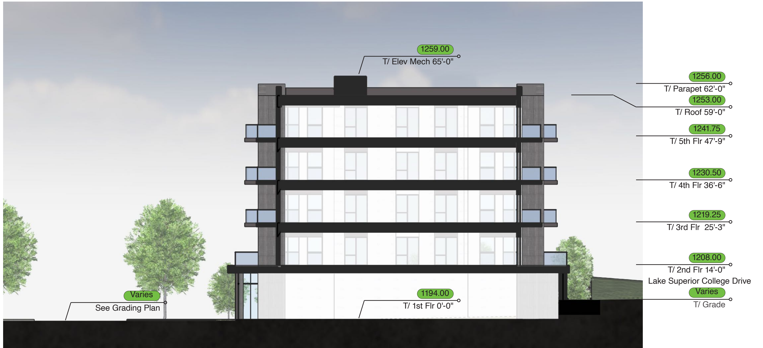
Section Through N/S - Looking West
